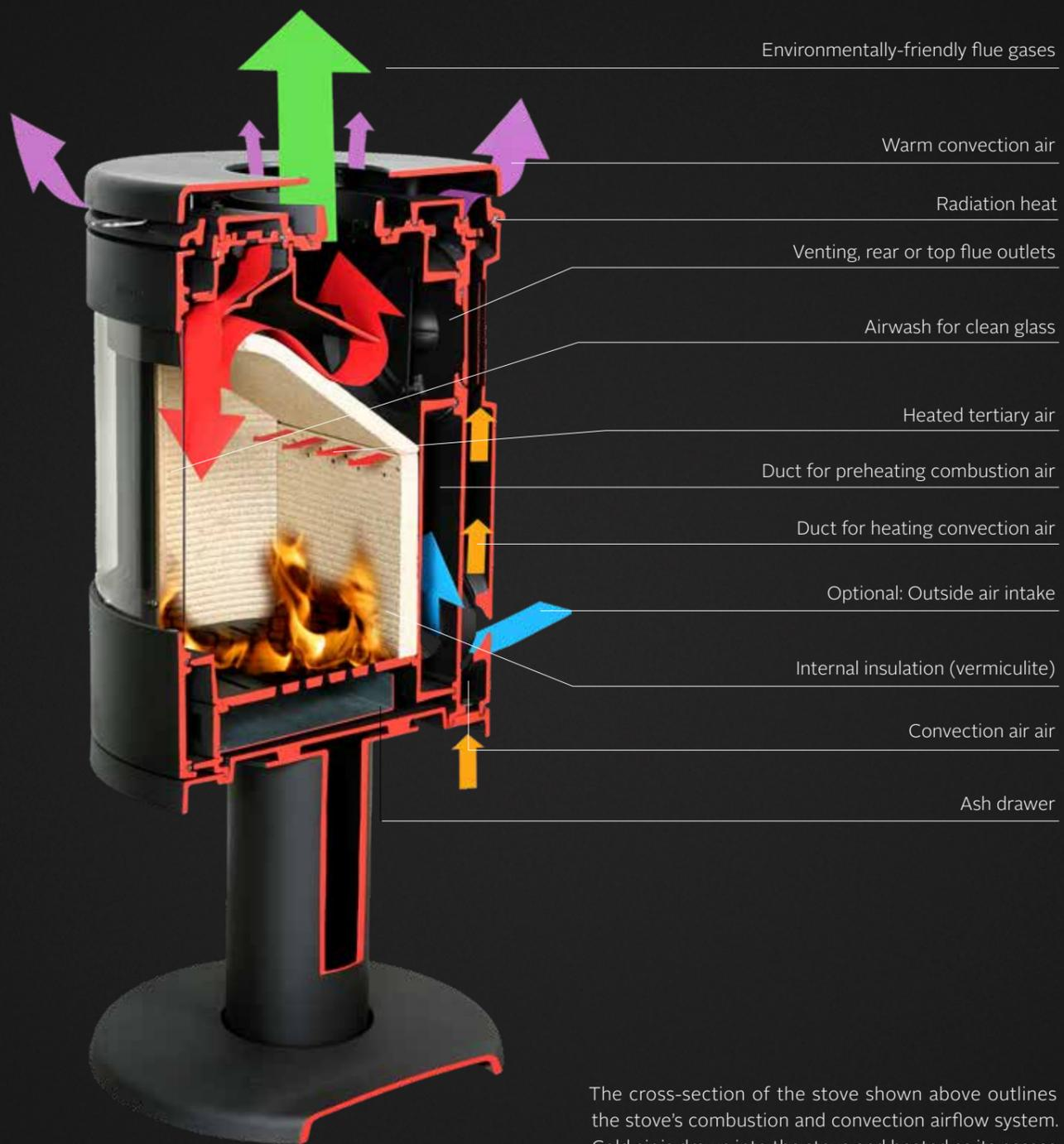
The cross-section of the stove shown above outlines the stove's combustion and convection airflow system. Cold air is drawn into the stove and heated as it passes through the cast iron channels (the heated air washes the glass keeping it clean, clear and free from soot). The hot air also provides perfectly heated combustion air (in addition the heated tertiary air aids secondary combustion of any smoke and gasses, increasing efficiency and reducing the environmental impact).
